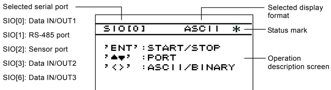
When no data is displayed, check the connection and the setting of the serial port.
