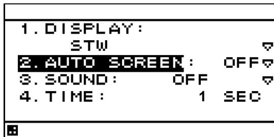
6. Select "ON" or "OFF" under "AUTO SCREEN" by using
