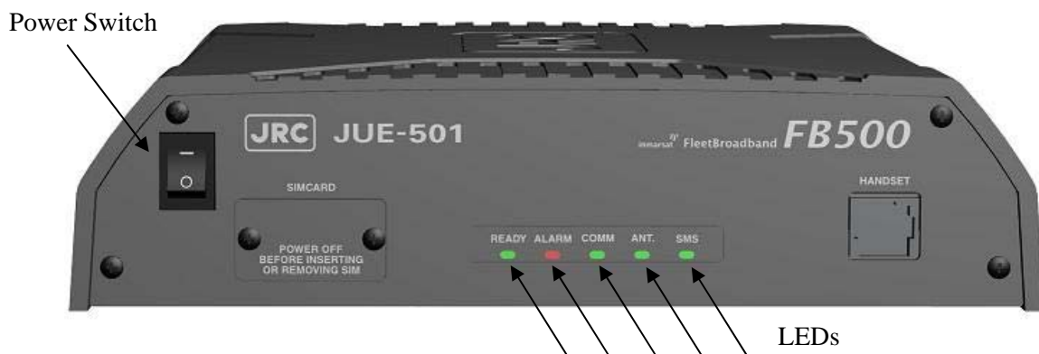
Fig.4.1.3a Power switch and LEDs of Main unit
